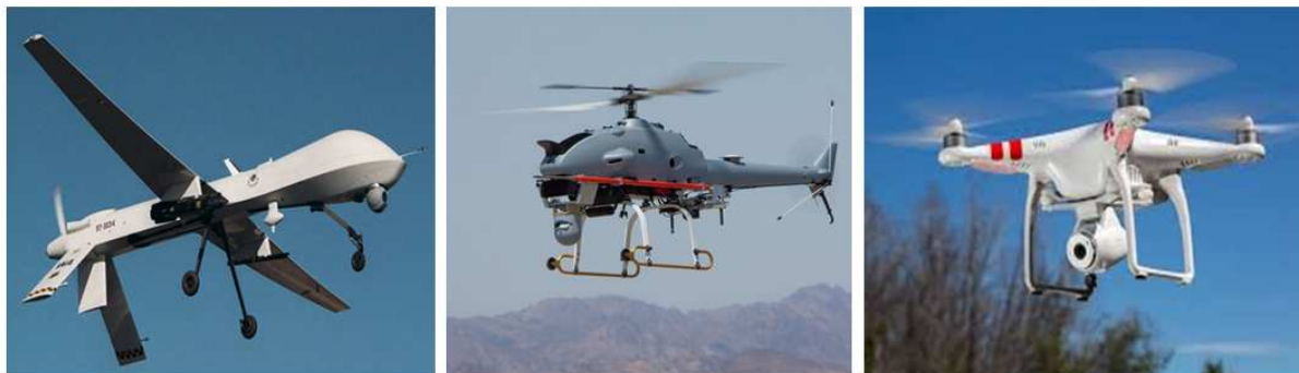
FIGURE 1.1: Three types of UAV: fixed-wing, rotary-wing, multi-rotor.
